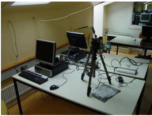
Figure 6.1. Workstation for animation, including: tripods, camera (pointing downward), FireWire cable, and PC. The tabletop is the work space for shooting objects placed under the camera.
