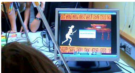
Figure 8.10 (Still 4.01). A bar on the computer screen indicates that the camera is shooting a frame, saving it and transferring the image to the Stop Motion Pro software.
